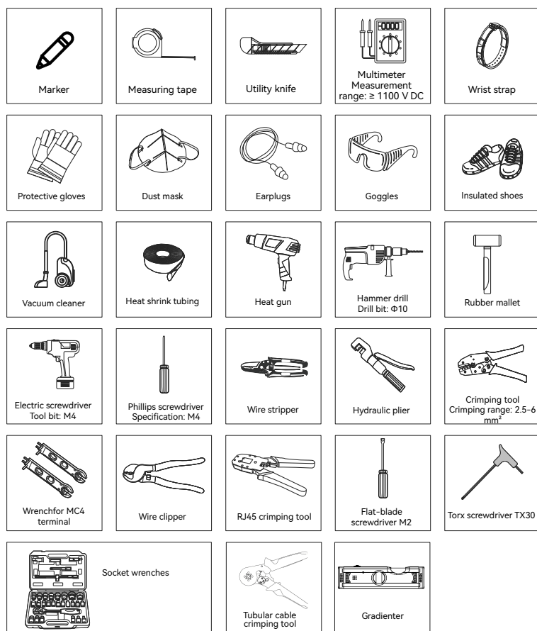
Figure 2.1. Suggested installation tools
